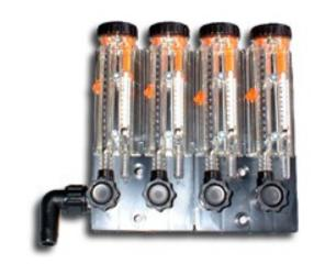
An adjustable sliding marking in form of an arrow indicates the desired value after an interruption. Easy cleaning. By unscrewing only one cover, the measuring housings can be simply cleaned by means of supplied brush.
